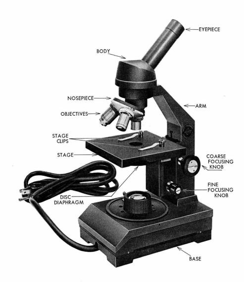
PARFOCAL—A term applied to objectives and eyepieces when practically no change in focus has to be made when one power is substituted for another. The objectives on your SWIFT Series M2240 are parfocalized at the factory so that only a slight turn of the fine adjustment is required when a change is made from low to a higher power.
