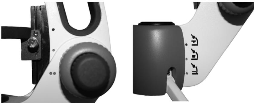
For proper stage ring adjustment, loosen the stage position thumbscrew to raise or lower the stage ring housing to line up with the desired stage position indicator marks. Tighten the thumbscrew to secure the stage
